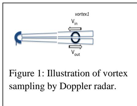
Figure 1: Illustration of vortex sampling by Doppler radar.
